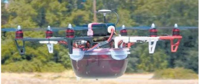
The model has six arms each with a motor and propeller. The red bowl on the bottom is a "Tupperware" like food storage container. Inside is a small video camera and a mobile phone. The mobile phone was tracking GPS coordinates of the flight path.
